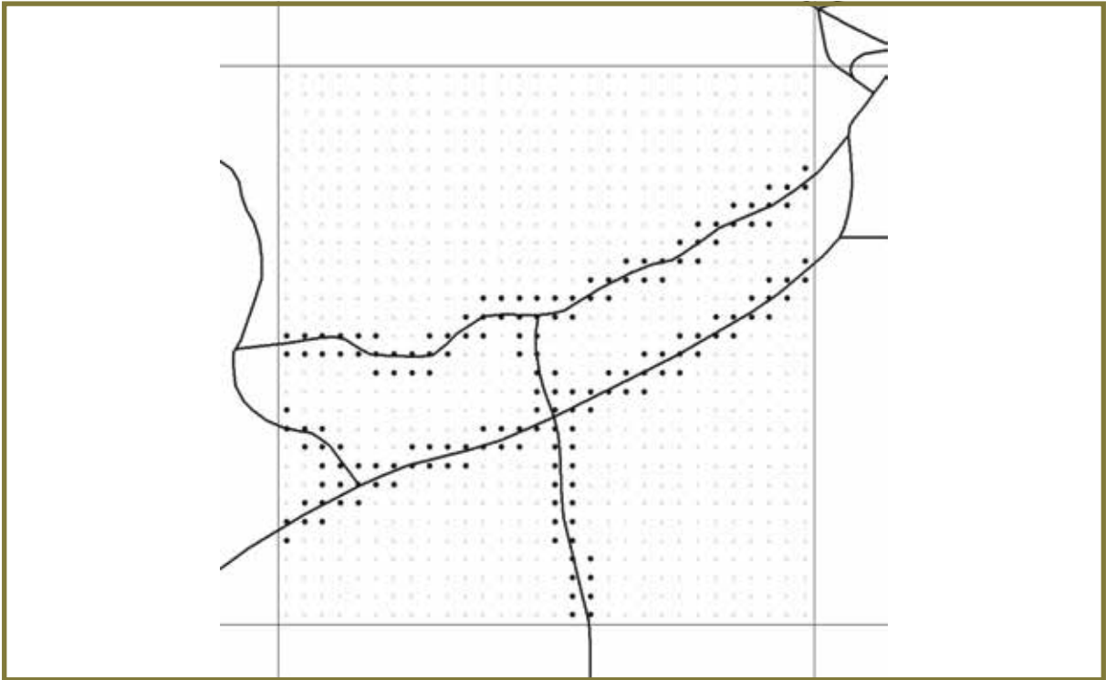
FIGURE 24. SAMPLE OF POINTS FOR A SURVEY ALONG THE ROAD BY SAMPLING LARGE SQUARE SEGMENTS.
