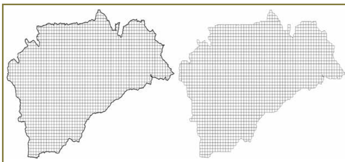
FIGURE 2. A SQUARE GRID ON AN ADMINISTRATIVE REGION. RIGHT: SQUARE GRID AFTER ELIMINATING SMALL GRID CELL PIECES.
